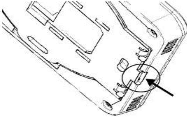
To detach the panel from the mounting surface, insert a flat object such as a screwdriver into the indicated slot of the mounting frame. This opens the clips of the mounting frame and allows the panel to be detached.
