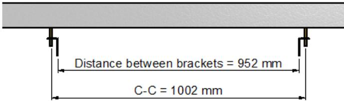
If so, then use the suspension brackets as jigs for the bolts so that the distance between brackets will be correct.
