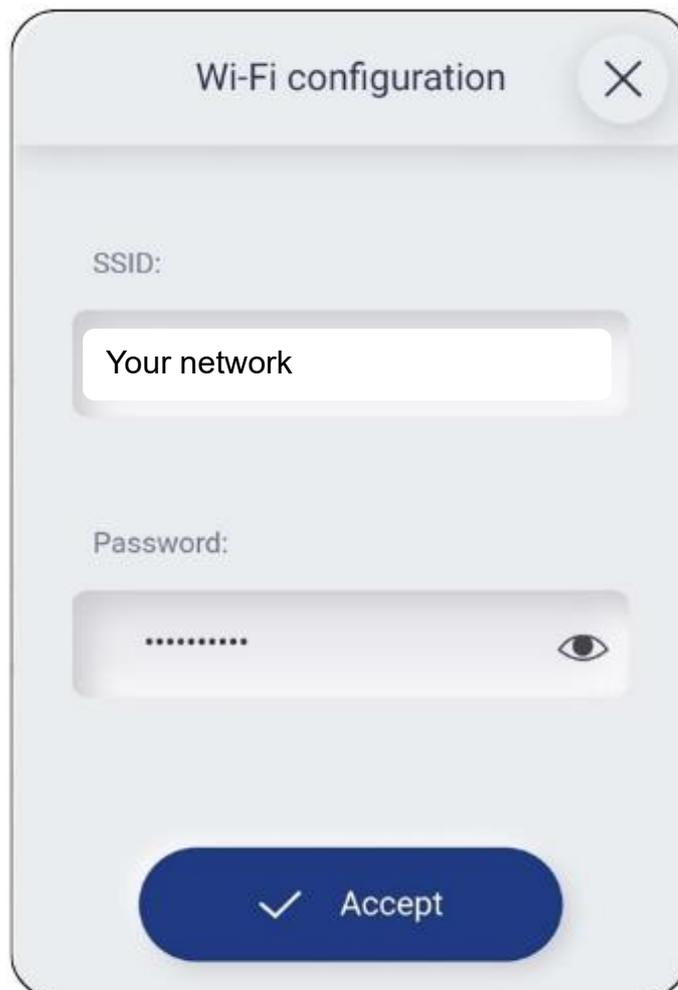
11. Once the network data has been entered correctly, the module automatically switches to Wi-Fi mode. To repeat the process, switch the module back to BY mode by holding down the ON/OFF button for 5 sec.
