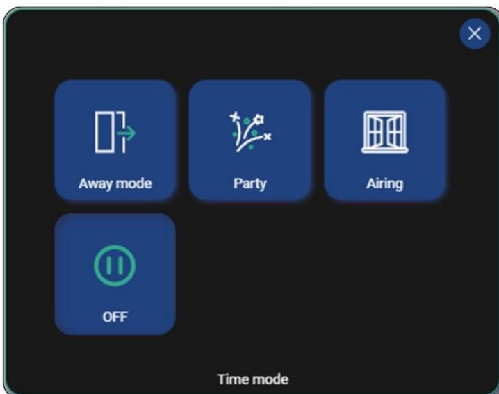
**Away mode** – Stops the operation of the unit, this mode can be used when the user leaves the room. The settings of this mode allow you to specify the duration.
