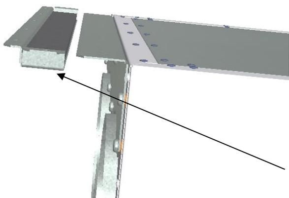
Attach one of the ceiling brackets in the correct position in the roof.
