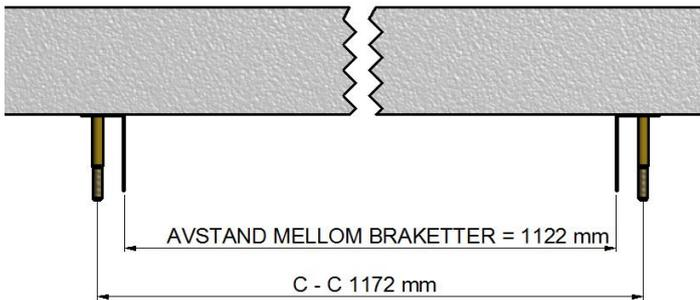
Use correct drill for use for the M10 mm expansion bolts.
