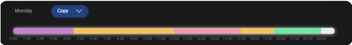
To copy the settings of a day, press the **Copy** button, then select the days to which you want to copy the settings in the drop-down menu and confirm.
