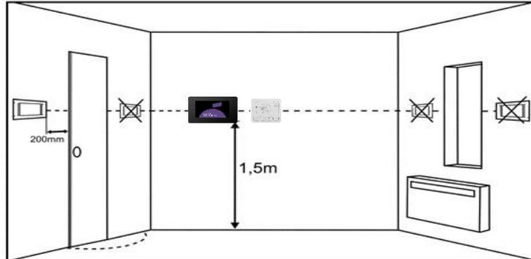
In order to reduce interference of temperature measurement by the panel, it is necessary to avoid places with strong sunlight, poor air circulation, close to heating devices, directly next to doors and windows (typically at least 200 mm from the edge of the door).
