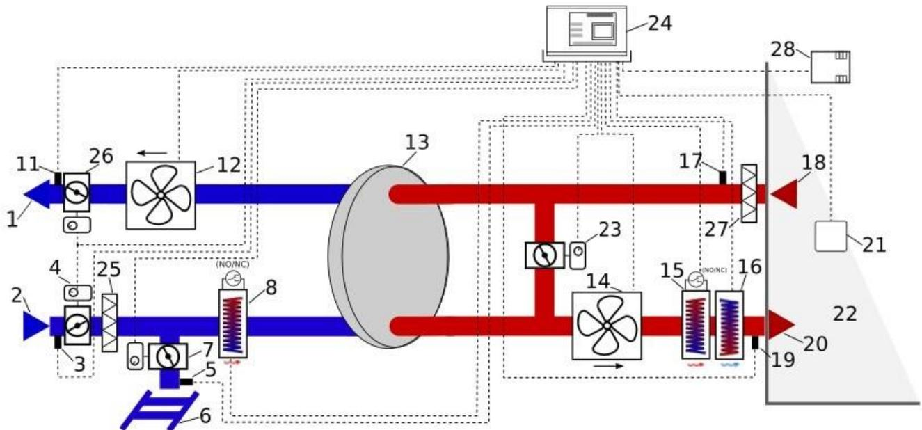
Ventilation scheme with a rotary exchanger and secondary cooler with freon or water, and primary and secondary electric heaters.
