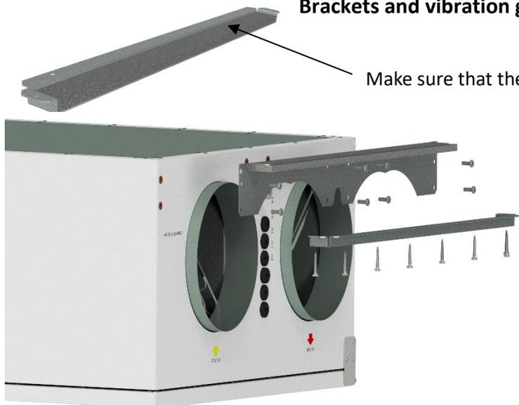
Suspension brackets screwed on the unit as shown on both ends of the unit.
