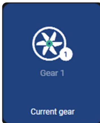
When pressed, it develops the current running mode selection screen, which allows to change the main operation mode, which is gears 1 (minimum), gear 2 (normal), gear 3 (maximum) and consequently the ventilation intensity and to stop the unit air operation.
