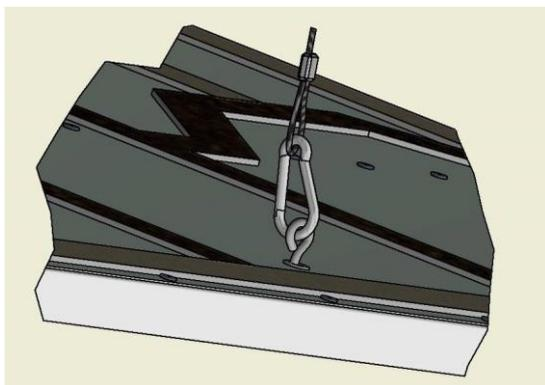
To close, after putting the hatch back on place, turn the latches the opposite way. You may use some pressure towards the hatch to close it.
