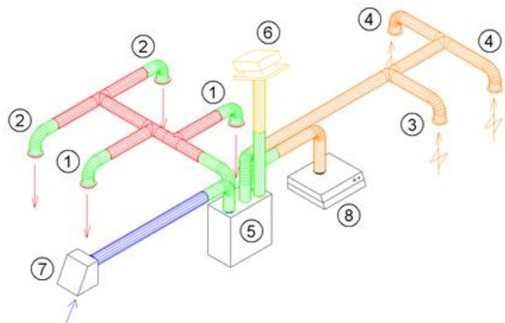
Instead of separate roof cowl for exhaust air and wall grid for fresh air there also can be used combi grids with inlet and outlet air are in the same box.
