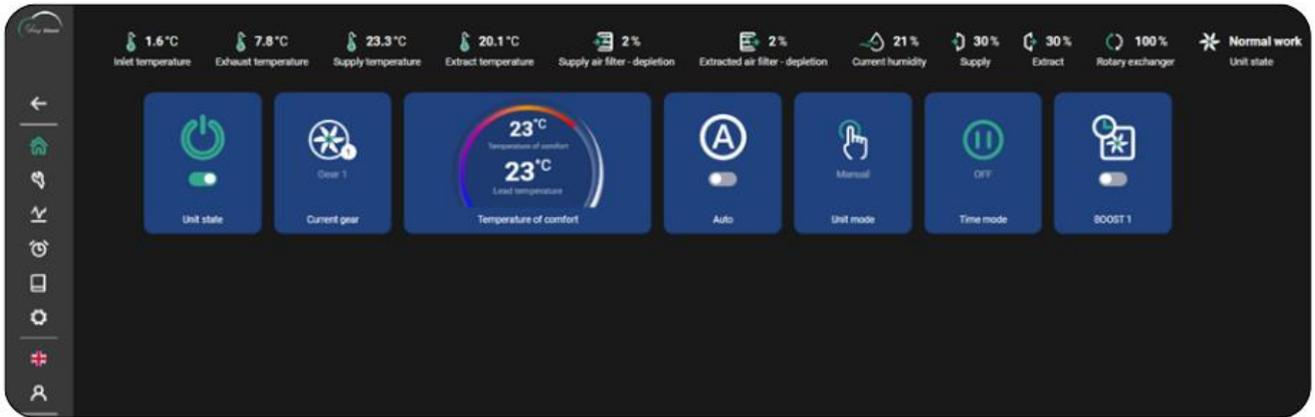
**Status of the control panel** - Enables the unit to be switched on/off.
