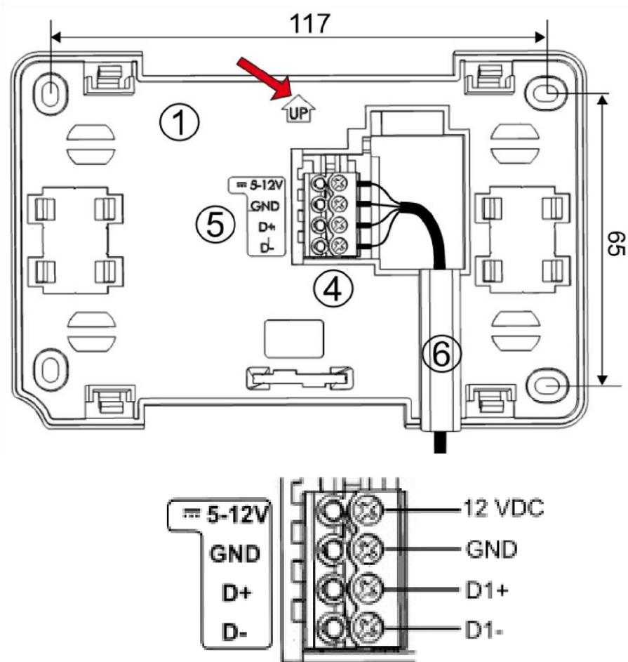
Drill holes in the wall and fix the mounting frame at the desired point on the wall with screws, keeping it in the correct position (UP). Then fix the panel to the mounting frame using the clips.
