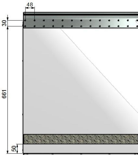
Glue vibration gasket to the back of the unit, see illustration. Approx. 50mm from the bottom of the unit.
