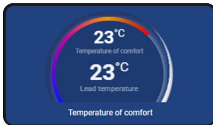
When the cursor is positioned over the tile, it will change its appearance to allow the values to be edited. It is possible to edit the comfort temperature using the “+” and “-” signs. The modification must be confirmed using the purple button in the bottom right corner of the tile.
