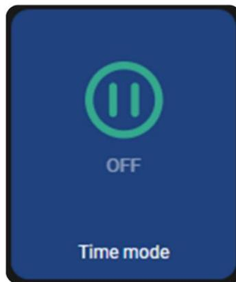
It enables the activation of a timed mode forcing a temporary change in fan control according to the settings of the mode. When pressed, it develops the time mode selection screen.
