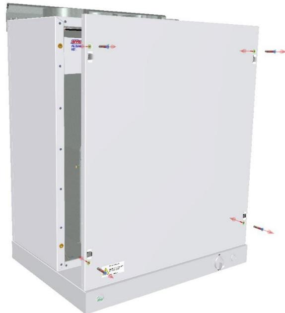
When hatch is mounted back on the unit, try to use almost same torque on all 4 screws.
